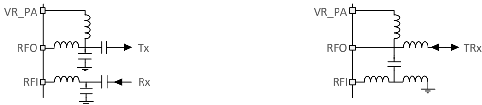
Figure 3. Individual RF transmit and receive paths (left) provides better sensitivity than the single shared TRx path (right).
